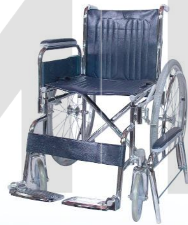
BS-7003 可折轮椅 Folding Wheel Chair 钢管车架、可拆扶手、可拆脚、电镀车架、PVC座垫、8寸塑胶前轮、24寸钢丝后轮 Description: Steel tube frame, detachable armrest, detachable feet, plating frame, PVC seat back cushion, 8 inch plastic front wheel, 24 inch wire rear wheel.
